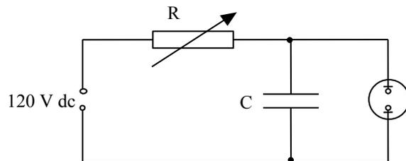
The neon lamp requires a potential difference of  $100\text{ V}$  across it before it conducts and flashes. It continues to glow until the potential difference across it drops to  $80\text{ V}$ . While lit, its resistance is very small compared with the resistance of  $R$ .
