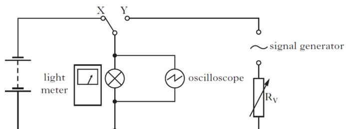
The switch is connected to X and the voltage across the lamp is 2.30 V. the reading on the light meter is recorded. The switch is now connected to Y. The resistance of  $R_v$  is adjusted until the light meter reading is the same as before.
