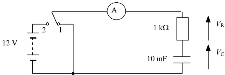
The switch is in position 1 and the capacitor is uncharged.
