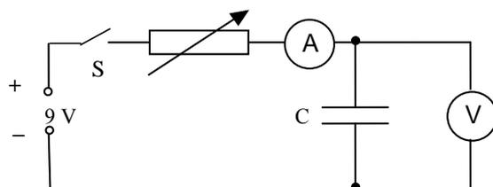
Switch S is now closed. By carefully adjusting the variable resistor R a constant charging current of 1.0 mA is maintained. The reading on the voltmeter is recorded every 10 seconds. The results are shown in the table below.
