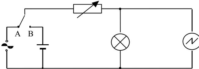
The variable resistor is used to adjust the brightness of the lamp until the lamp has the same brightness when connected to either supply.
