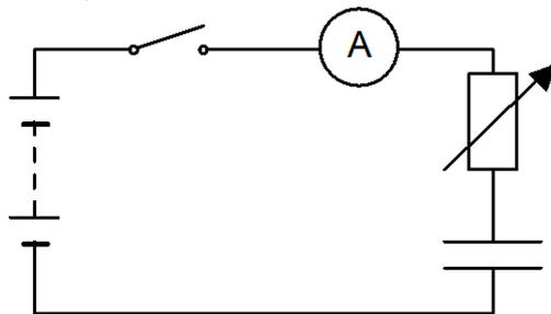
The capacitor is initially uncharged. The switch is now closed.
