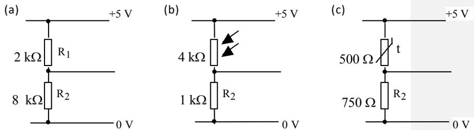
21. Calculate the p.d. across AB (voltmeter reading) in each of the following circuits.
