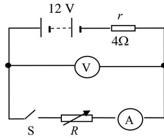
For each setting of the variable resistor the current in the circuit is recorded.
