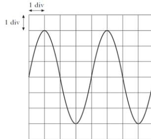
The time-base is set at 0.01s/div and the y-gain is set at 4.0 V/div.
