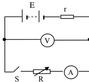
The variable resistor provides known values of resistance  $R$ .
