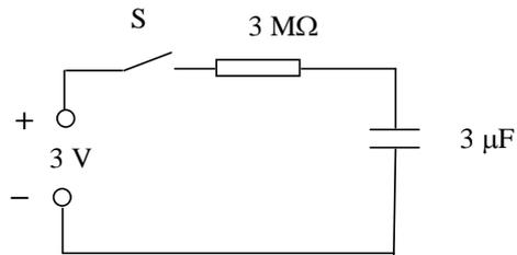
The power supply has negligible internal resistance. The capacitor is initially uncharged.
