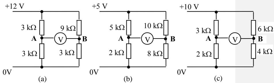
22. A circuit consisting of two potential dividers is set up as shown.
