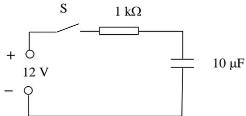
The capacitor is initially uncharged.
