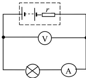
The current in the lamp is  $0.20\text{ A}$  and the reading on the voltmeter is  $3.0\text{ V}$ . Calculate the internal resistance of the battery.
