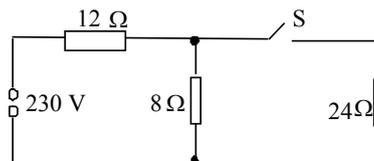
Calculate the current in each resistor when:
