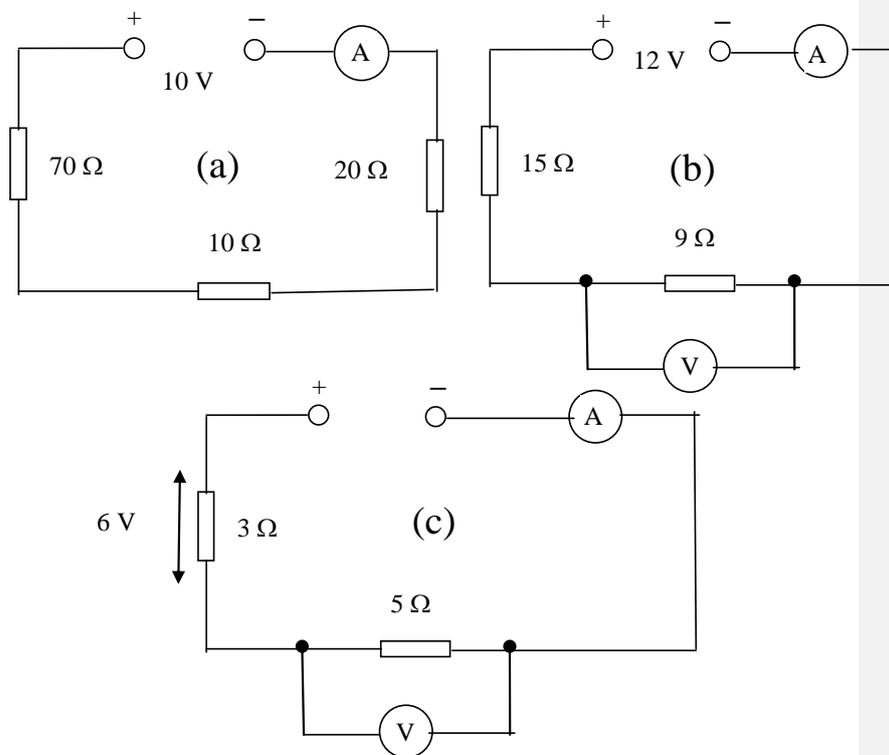
6. Calculate the unknown values  $R$  of the resistors in the following circuits.
